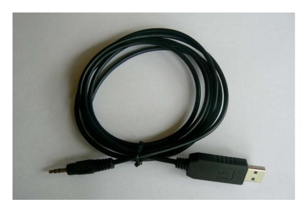
This is the exact equivalent to the 1.8m USB to 3.5mm stereo plug cable available from PICAXE. It uses the same miniature FT232R chip moulded into the USB connector and has the identical pinout for connection to a 3.5mm stereo socket.
